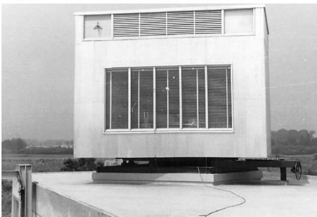
Fig3 Revolving Type of Air Conditioning Test Room at Obayashi Corporation in Kiyose, Tokyo
